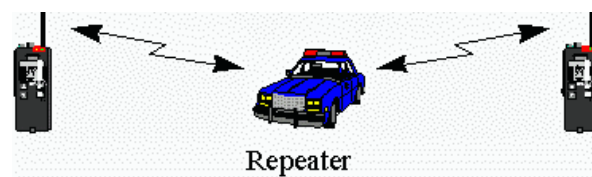
Abbildung 8: Direct Mode Repeater Operation
